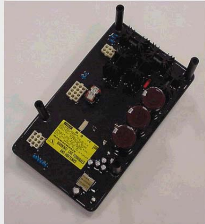
Caterpillar Digital Voltage Regulator or “CDVR”
